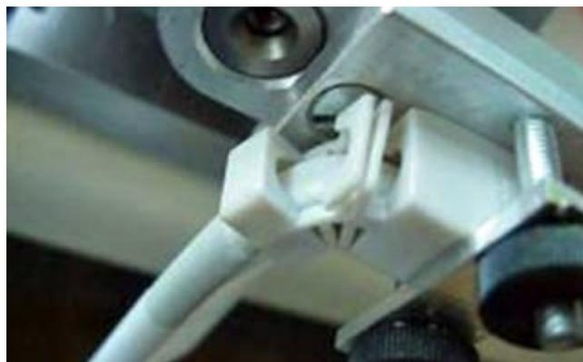
Alternative bend protection broken without protective effect
