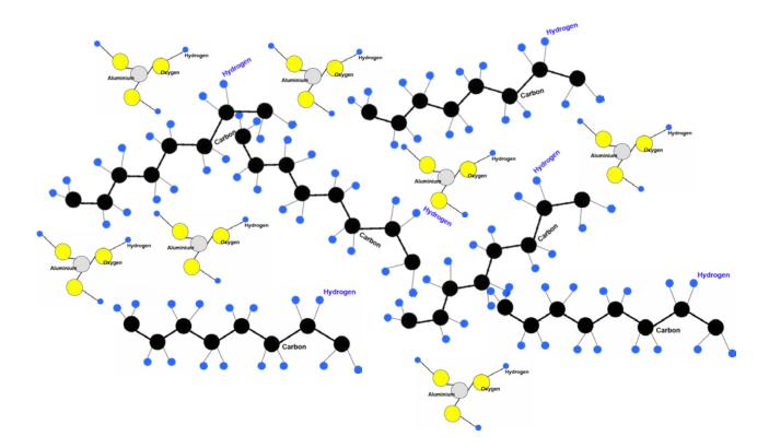
The basic plastic, polyethylene PE, is mixed with the additive. The additive decomposes when energy is supplied (fire) and withdraws energy from the system (burning plastic), which is necessary for the propagation of the chemical reaction (fire).
