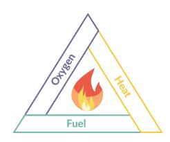
If one of the three elements, oxygen, combustible material or heat (energy) is extracted from a fire, the flame suffocates. In the case of self-extinguishing materials, the heat (energy) of the fire starts a so-called endothermic (endotherm = energy consuming) chemical reaction, that withdraws energy and thus heat from the fire (analogous to extinguishing a fire with water).
