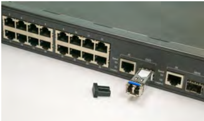
030.6125 SFP transceiver plugged into an switch port
